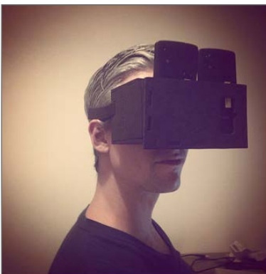
Figure 2. Google Cardboard-based HUD with two phones, providing stereoscopy.
